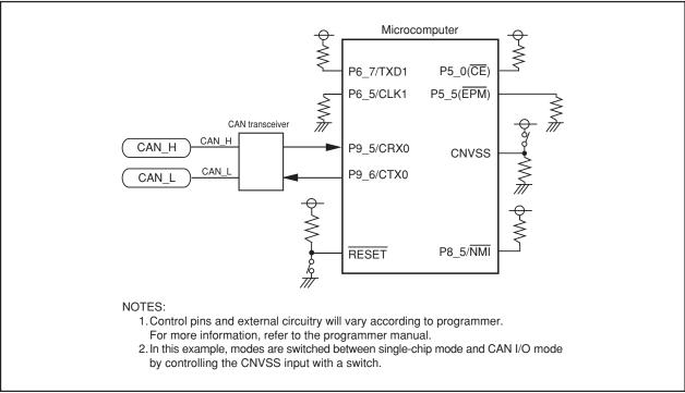
Figure 20.19 Circuit Application in CAN I/O Mode
